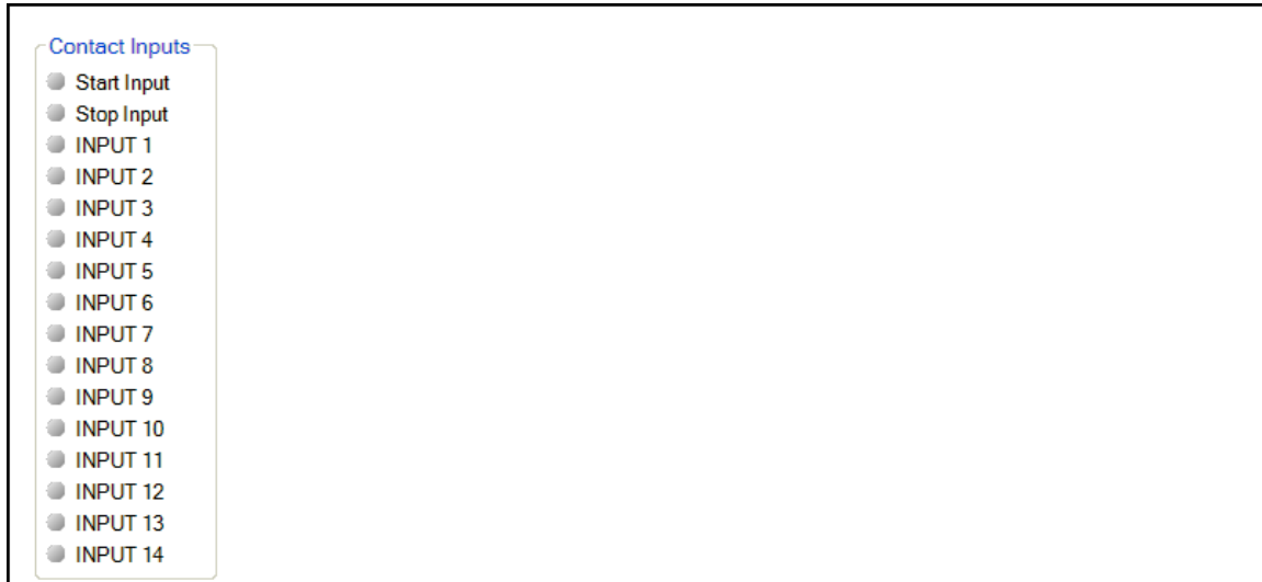
Figure 13-14. DECS-250 Contact Inputs Status Indication Screen
