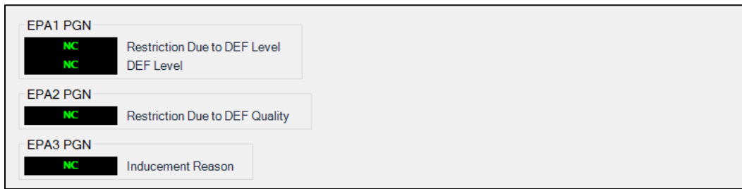
Figure 3-29. Metering Explorer, J1939 ECU, Deutz Status
