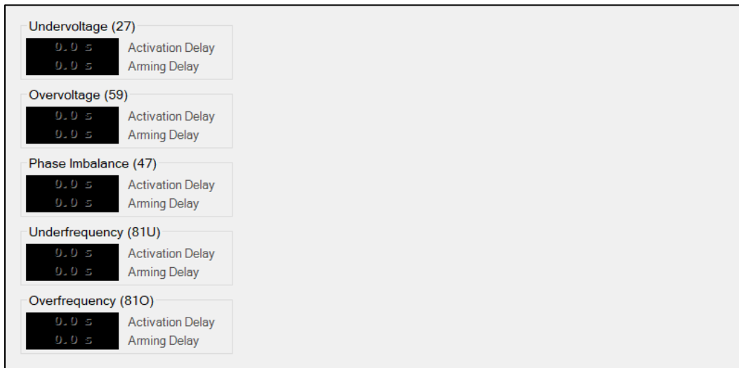
Figure 3-16. Metering Explorer, Timers, Generator Protection Timers
