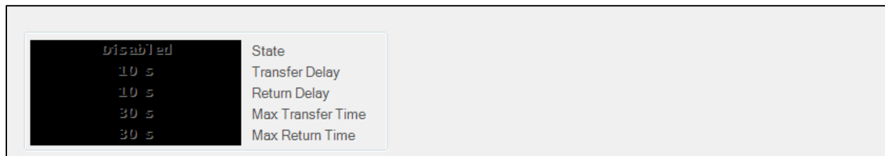
Figure 3-36. Metering Explorer, Mains Fail Transfer Status
